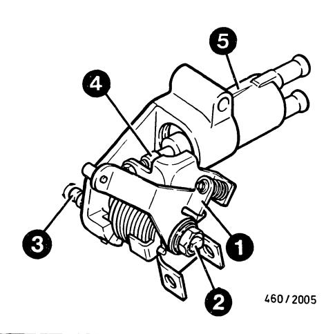
As the engine warms up, the lifting rod moves against the pre-tensioned KSB lever and turns the eccentric in a counter-clockwise direction.
